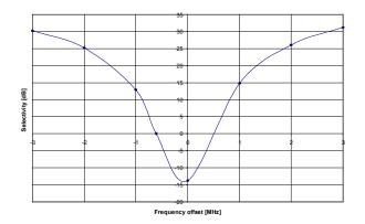
Figure 59: Typical Selectivity at 500 kBaud. IF Frequency is 307.4 kHz. MDMCFG2.DEM\_DCFILT\_OFF=0
