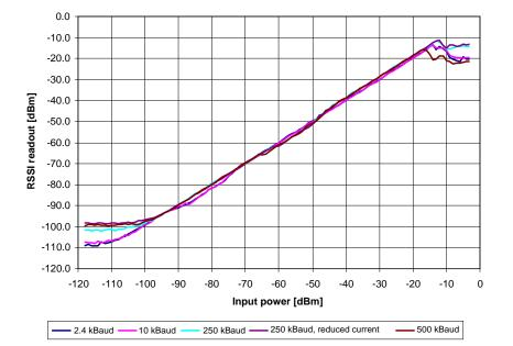
Figure 52: Typical RSSI Value vs. Input Power Level for Some Typical Data Rates
