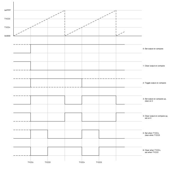
Figure 32: Output Compare Modes, Timer Free-running Mode
