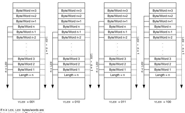
If  $n \ge \text{LEN}$ , LEN bytes/words are being transferred. The dotted line shows the case where LEN = n + 1
