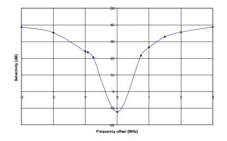
Figure 58:Typical Selectivity at 250 kBaud. IF Frequency is 457 kHz. MDMCFG2.DEM\_DCFILT\_OFF=1
