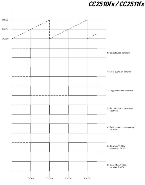
Figure 33: Output Compare Modes, Timer Modulo Mode
