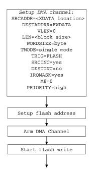
Figure 21: Flash Write using DMA
