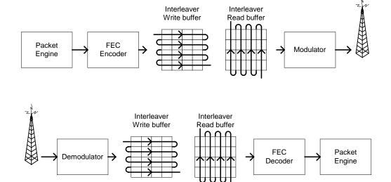
Figure 53: General Principle of Matrix Interleaving
