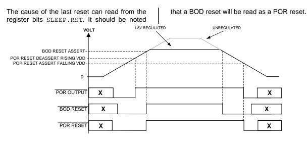
Figure 19: Power-On-Reset and Brown Out Detector Operation
