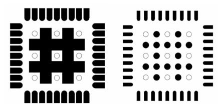
Figure 13: Left: Top Solder Resist Mask (negative). Right: Top Paste Mask. Circles are Vias.
