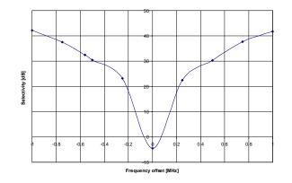
Figure 55: Typical Selectivity at 2.4 kBaud. IF Frequency is 273.9 kHz. MDMCFG2.DEM\_DCFILT\_OFF=1
