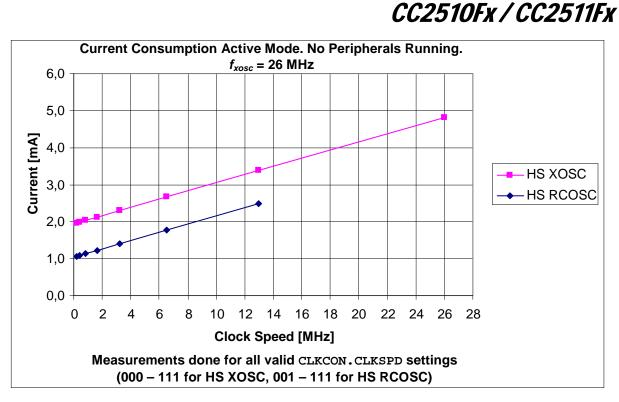
Figure 1: Current Consumption (Active Mode) vs. Clock Speed
