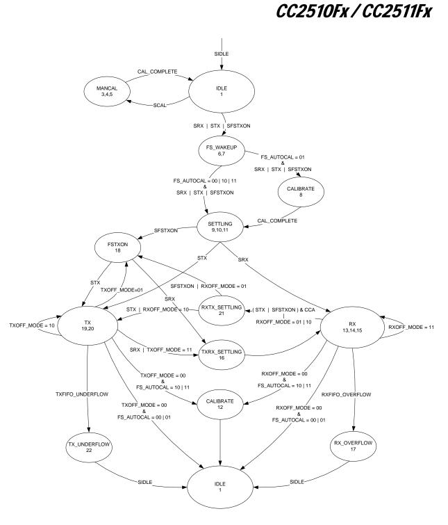
Figure 54: Complete Radio Control State Diagram
