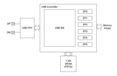
Figure 43: USB Controller Block Diagram
