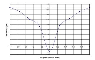
Figure 56: Typical Selectivity at 10 kBaud. IF Frequency is 273.9 kHz. MDMCFG2.DEM\_DCFILT\_OFF=1
