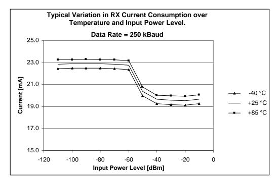
Figure 2: Typical Variation in RX Current Consumption over Temperature and Input Power Level. Data Rate = 250 kBaud.
