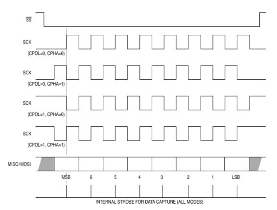
Figure 41: SPI Dataflow
